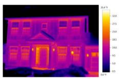
Infrared image of building envelope energy loss
