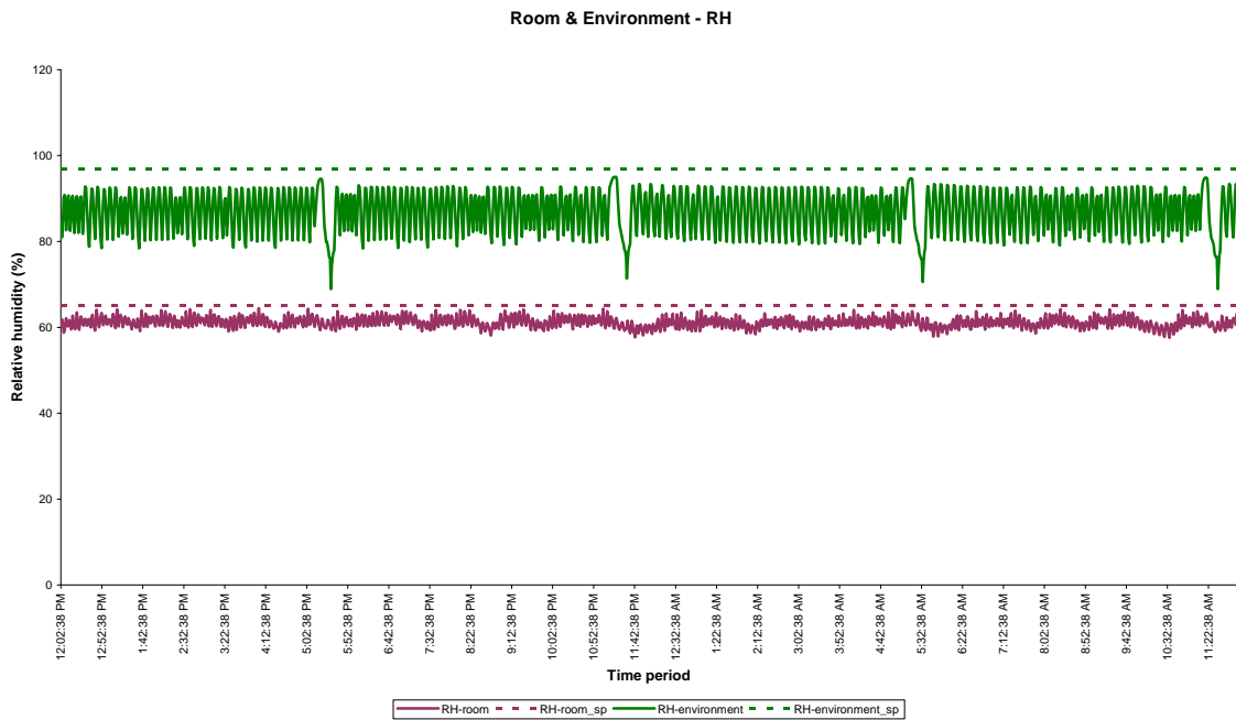
Figure B-27: Relative humidity of the room and environmental side during S1-Alt3
