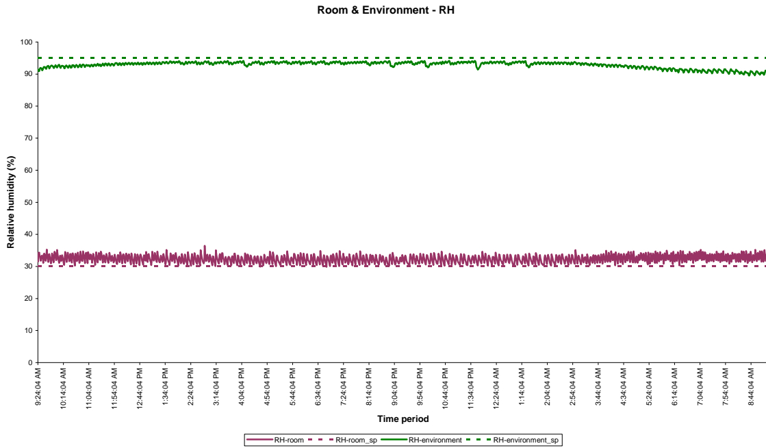
Figure B-144: Relative humidity of the room and environmental side during C1-Alt8
