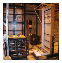
Test Set-up: Airflow Chamber
