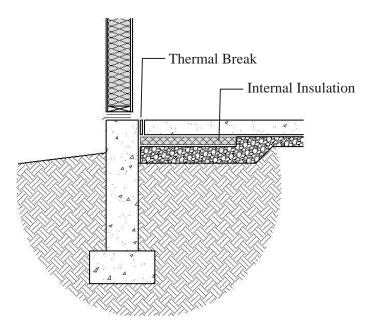
Figure PA 302.8 (2) Interior Slab Insulation
