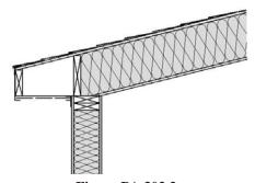
Figure PA 302.2 Ceiling Without Attic Spaces
