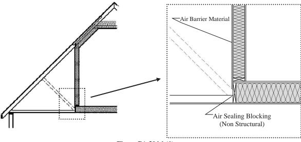
Figure PA 304.1 (1) Air Sealing—Knee Walls
