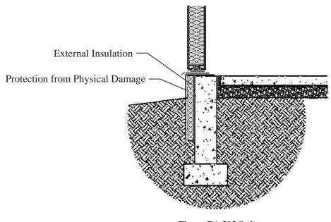
Figure PA 302.8 (1) Exterior Slab Insulation
