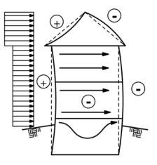
**Figure 1.** Wind creating pressure differentials across the building enclosure. Wind striking the house creates a positive pressure on the windward side and a negative pressure on the leeward side. Both positive and negative pressures create air leakage through cracks and holes in the building enclosure.
