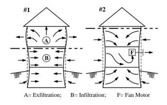
**Figure 2.** Air infiltration patterns with and without the operation of a kitchen exhaust system. Scenario #1 depicts the stack effect in a house under natural winter time conditions. Scenario #2 depicts how mechanical exhaust can alter the pressure pattern creating a negative pressure throughout the house.
