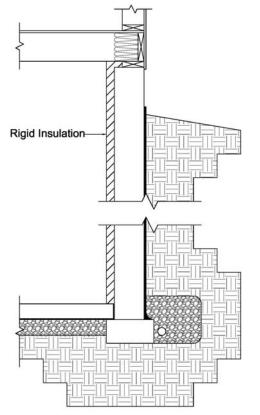
Installing foam board on the interior of the foundation provides a continuous layer of insulation. This limits thermal bridging yet makes running utilities difficult. Due to flame spread requirements, continuous foam board must be covered except for some foil-faced products.
