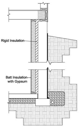
Combining continuous and cavity insulation systems offer a highly efficient basement wall. By installing a stud wall on the interior of the continuous insulation board, a finished system is provided. Thermal bridging is limited by the continuous layer but still is present. Thickness of the system becomes an issue.
