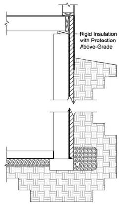
Exterior basement insulation systems provide a potentially habitable space to occupants. These systems can easily be converted to a habitable basement by installing a stud wall without any additional insulation. In general, basements with exterior insulation serve as well performing utility space with the option to finish.
