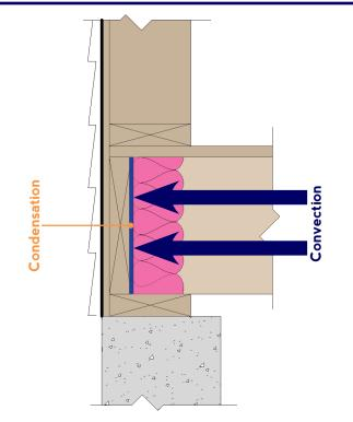
**Figure 2: Rim joist assembly w/fiberglass insulation** Fiberglass insulation provides thermal resistance to the assembly but does not prevent vapor through convection from condensing on the interior surface of the rim joist.
