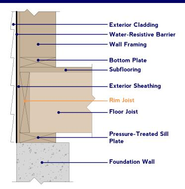
Figure 1: Uninsulated rim joist assembly
