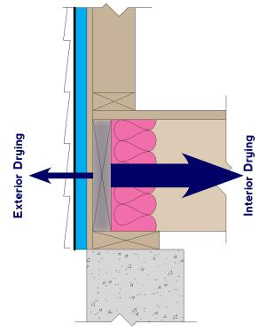
**Figure 4: Rim joist w/exterior foam insulation** Exterior foam insulation raises the temperature of the inside face of the rim joist to reduce the likelihood of condensation while still allowing drying to the interior.
