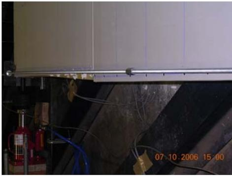
A photograph showing the edge of a drywall panel with a more significant gap from the metal stud. A fire extinguisher and blue cables are visible in the background. A timestamp '07.10.2006 15:00' is visible in the bottom right corner. |
