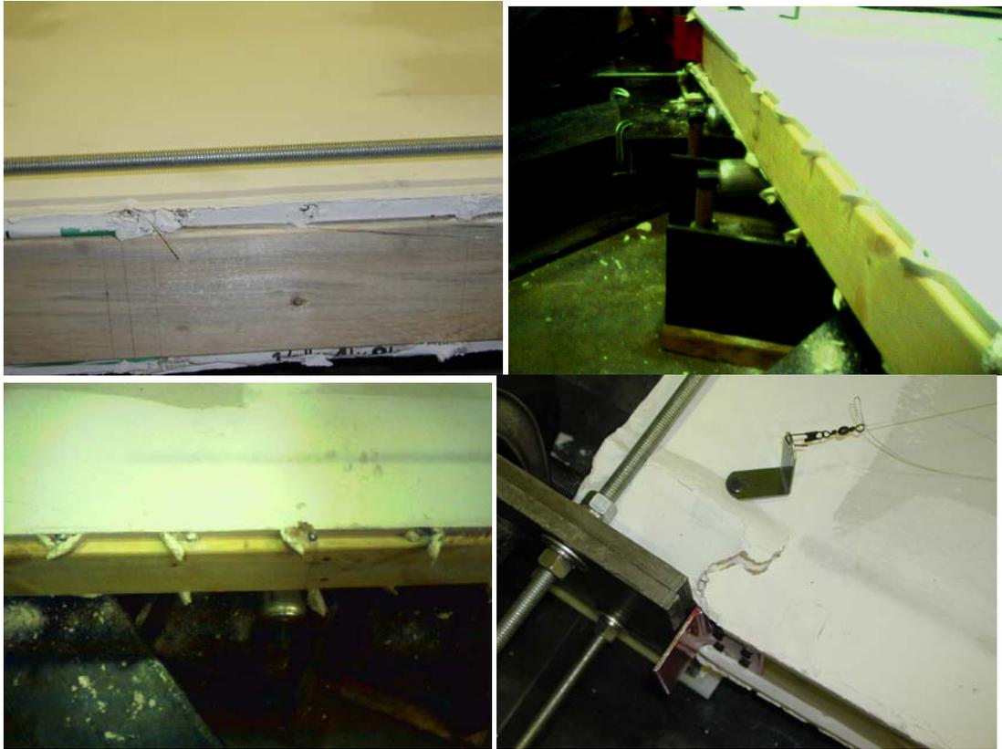
**Fig. 4-15: Failure modes for specimen WSFC1**
