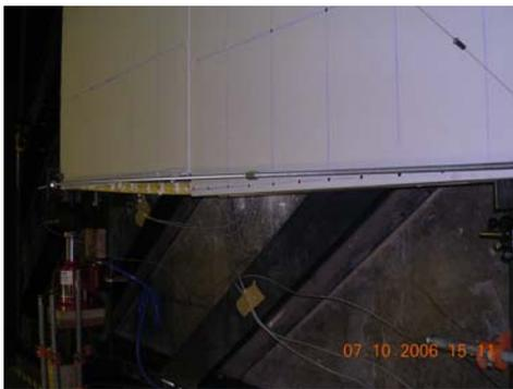
A photograph showing the edge of a drywall panel with a very large gap from the metal stud. A fire extinguisher and blue cables are visible. A timestamp '07.10.2006 15:11' is visible in the bottom right corner.                        |
