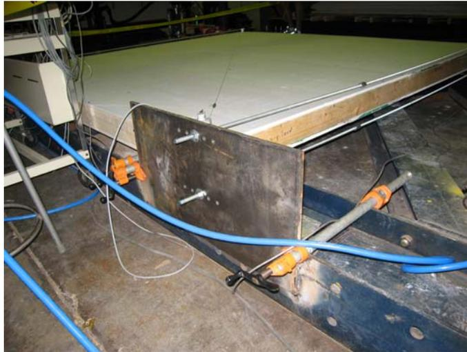
**Fig. 3-6: Steel plate holding the tie-rods at the bottom side of the specimen**
