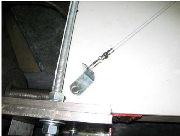
**Fig. 3-13: Detail of the tie-rod connection to steel plate**
