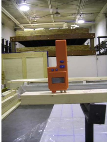
**Fig. 3-27: Moisture content measuring device**
