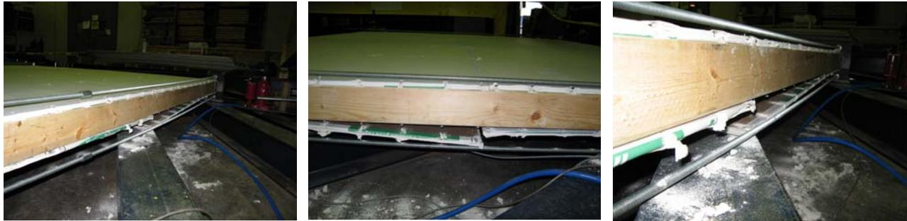
**Fig. 4-9: Three views of pull out separation of the drywall panel from frame**
