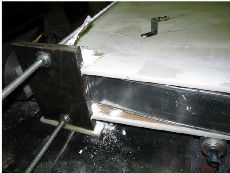
**Figure 4-41: Bending of Top Track of Steel Stud Wall**
