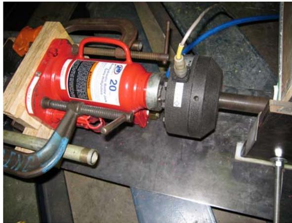
**Fig. 3-10: Load cell attached to each loading jack**
