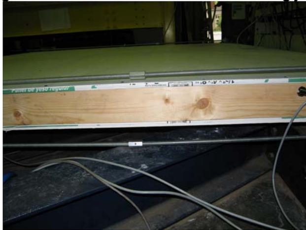
**Fig. 3-11: Tie rods attached on both sides of wall specimen**
