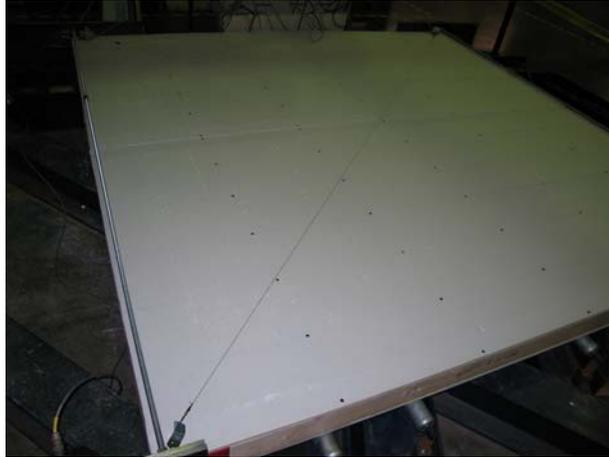
(b) Rollers placed under top-side of the wall specimen
