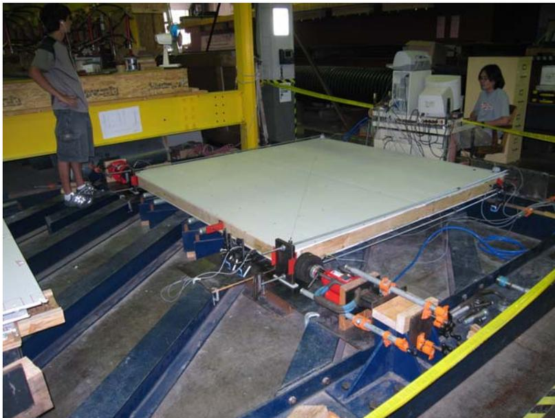
**Fig. 3-5: Position of a typical specimen on the test frame**
