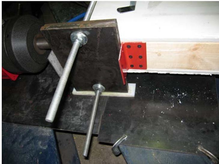
**Fig. 3-7: Steel plate holding the tie rod at top side of specimen**
