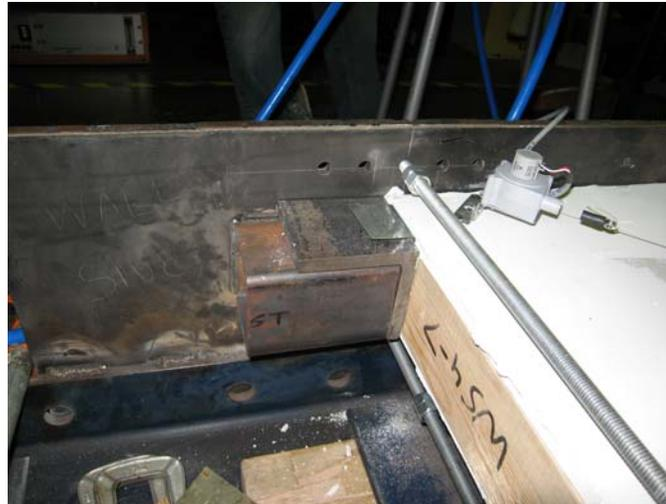
**Fig. 3-16: End stops at bottom steel plate to prevent sliding**
