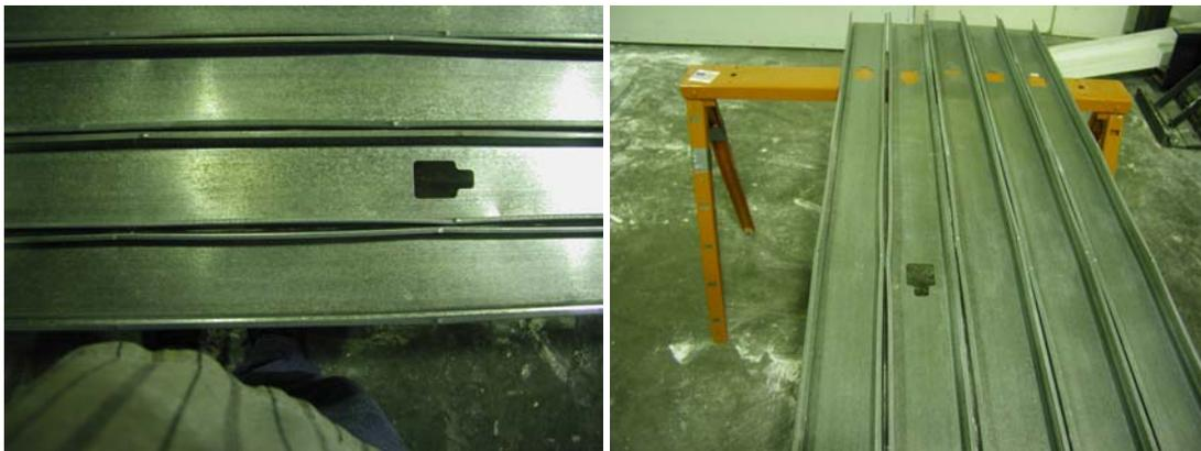
**Fig. 4-22: Specimen MSC1 damage-disassembled studs**
