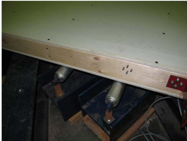
(c) Rollers placed under top-side of the wall specimen
