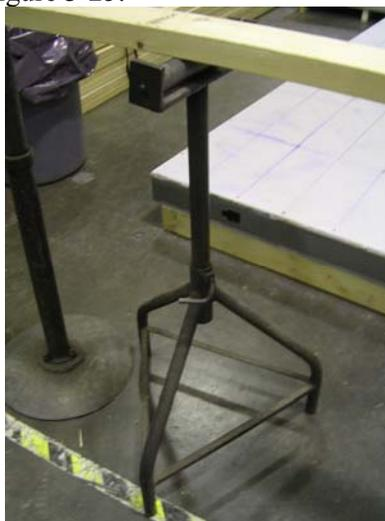
**Fig. 3-25: Simple support for E-test**
