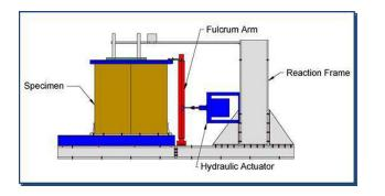
Additional in-plane and out-of-plane shear load testing, the Strong Floor and Reaction Frame is capable of applying over 400 kips of cyclic lateral load to various wall, frame, and slab assemblies. This facility can also be configured to perform gravity load testing on different types of framing systems and prism tests on masonry systems. Displacement, strain, rotation, pressure, temperature and flow
