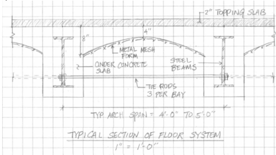
Figure 1: Typical Section of the Floor System
