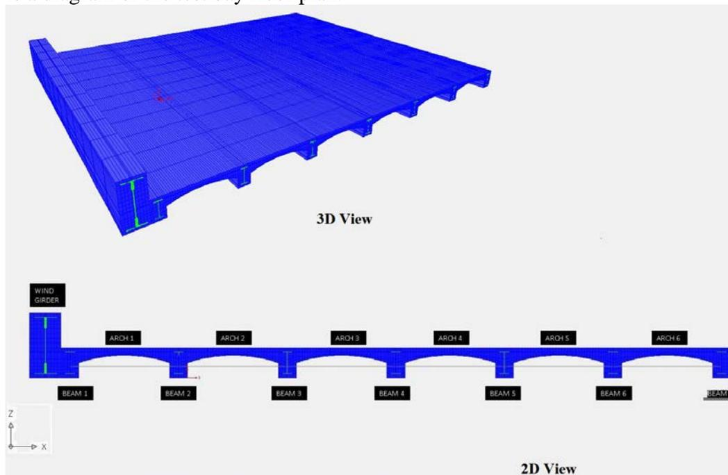
Figure 2: Analysis Model of the 28<sup>th</sup> floor test area
