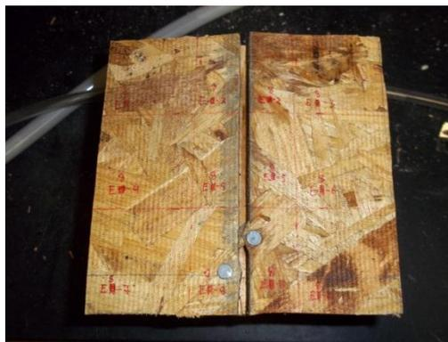
Figure 10: Sample with Vertical Joint (VJ)
