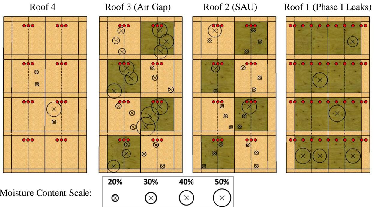
Figure 7: Maximum observed moisture contents in full-scale roofs
