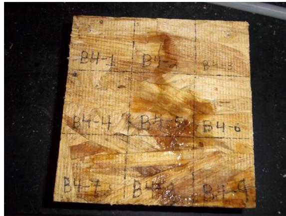
Figure 6: Nine subsections to each sample
