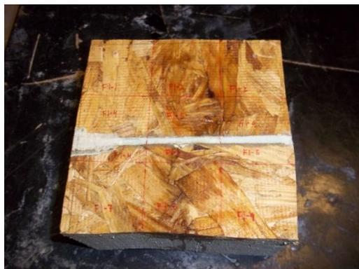
Figure 9: Sample with Horizontal Joint (HJ)
