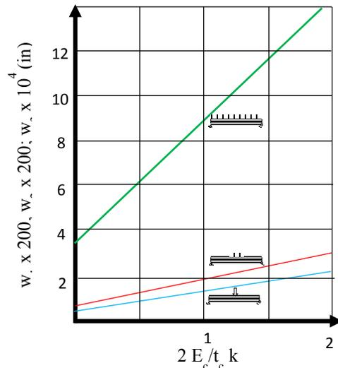
Fig. 11. Effect of  $E_c/t_c K$  on Maximum Deflection
