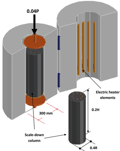
**Figure 6. Scaled-down fire test of a real-scale concrete**
