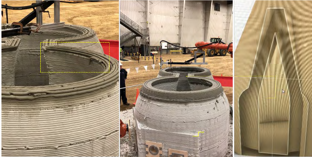
Figure 5: (Top) Physical experimentation of various edge configurations and the material deformation at the edges during robotic 3D printing. (Bottom) Failing of beads at interior side of tapering cone (marked in dotted yellow line). (Bottom right) Sectional view of module geometry at connector showing fillet edges
