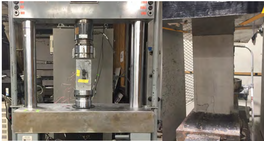
Figure 2. Universal testing machines used for applying axial compression loading to the samples
