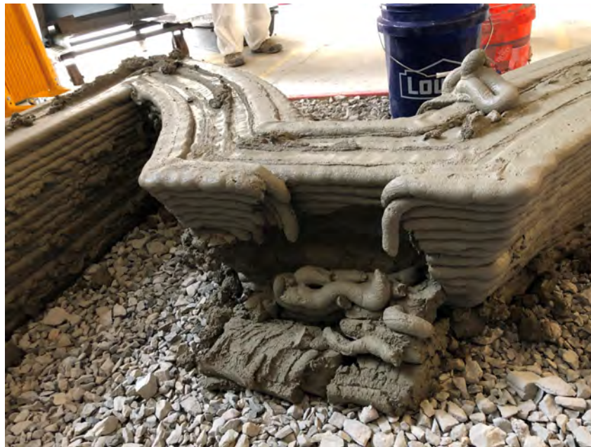
Figure 4: Physical experimentation of a sample concrete structure printed to test material deformation at 65-degree angle. The beads failing on the interior side can be seen.
