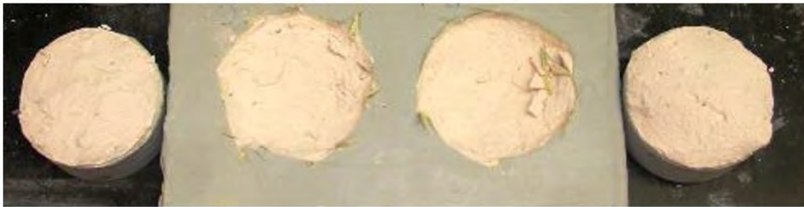
Figure 5: Pull-adhesion test result from a liquid-applied sheathing membrane/air barrier applied to a gypsum panel. Strong adhesion led to failure in the panel core.
