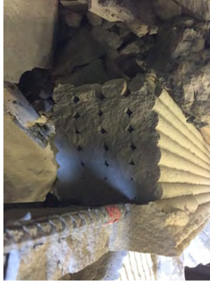
Figure 9. Voids in a 3D printed beam due to the material deposition process
