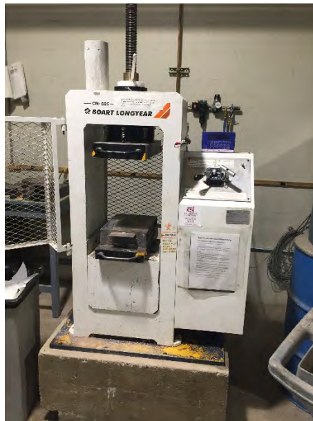
Figure 1. The material testing machine used to determine the ultimate strength of the samples: Boart Longyear loading frame Model CM-625 with a CSI Model CS-100-2A Retrofit with a Capacity of 400Kips
