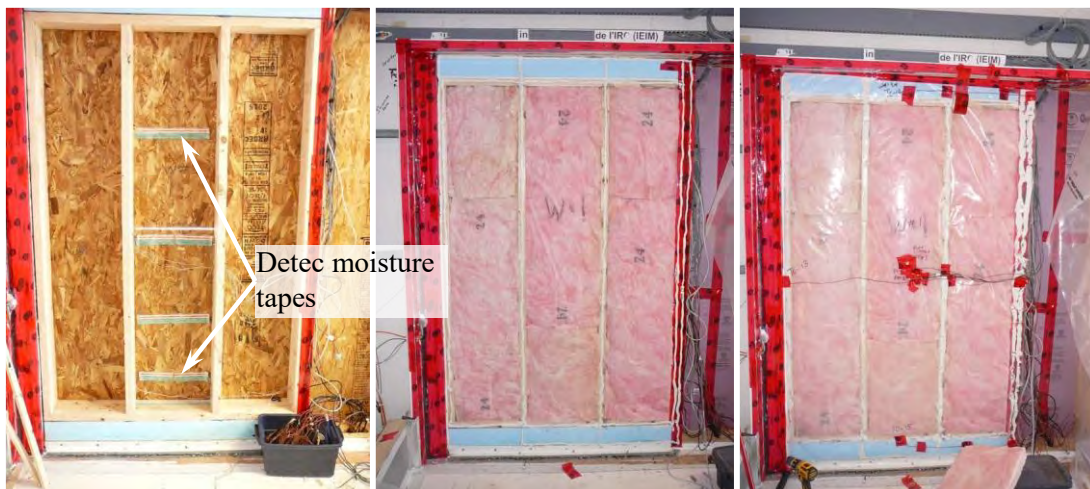
Figure 4. Example of wall specimen assembly construction showing locations of moisture detection tapes, temperature sensors and RH sensors
