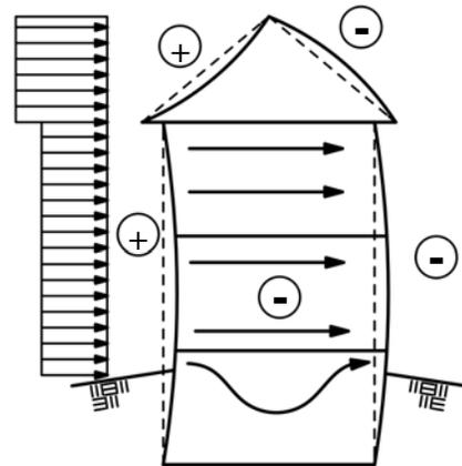
**Figure 1.** Wind creating pressure differentials across the building enclosure. Wind striking the house creates a positive pressure on the windward side and a negative pressure on the leeward side. Both positive and negative pressures create air leakage through cracks and holes in the building enclosure.
