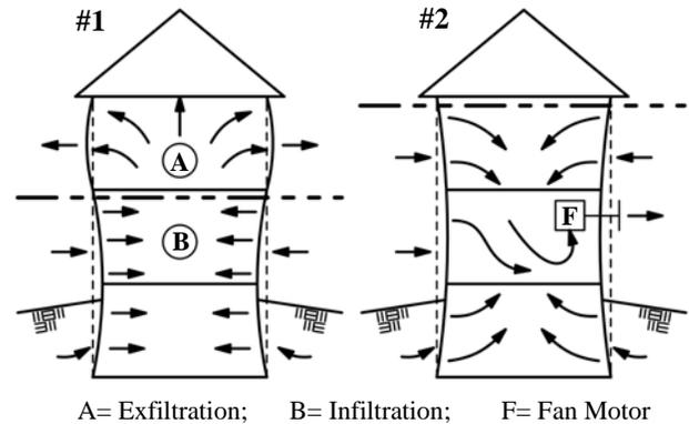
**Figure 2.** Air infiltration patterns with and without the operation of a kitchen exhaust system. Scenario #1 depicts the stack effect in a house under natural winter time conditions. Scenario #2 depicts how mechanical exhaust can alter the pressure pattern creating a negative pressure throughout the house.
