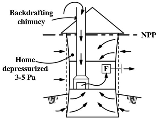
**Figure 3.** Certain levels of house tightness and exhaust rates may combine to create pressures high enough to cause the draft of combustion appliances to reverse.
