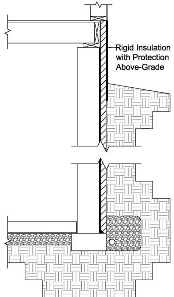
Figure 1: Exterior Insulation
