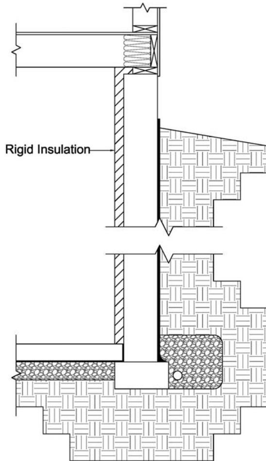
Figure 3: Interior Insulation
