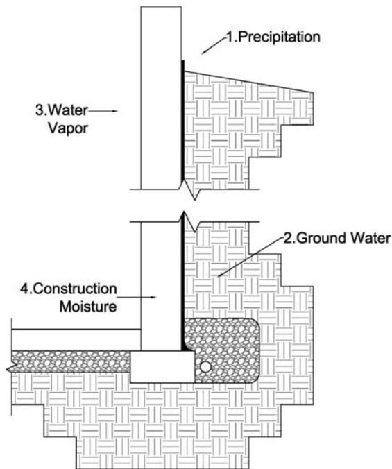
Figure 5: Moisture Sources for Below-Grade Walls
