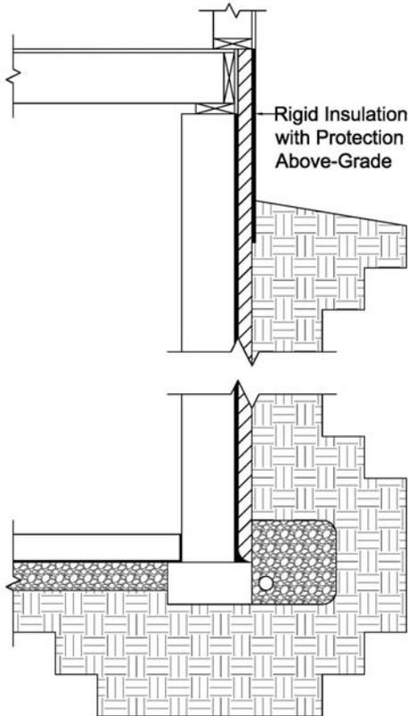
Exterior basement insulation systems provide a potentially habitable space to occupants. These systems can easily be converted to a habitable basement by installing a stud wall without any additional insulation. In general, basements with exterior insulation serve as well performing utility space with the option to finish.
