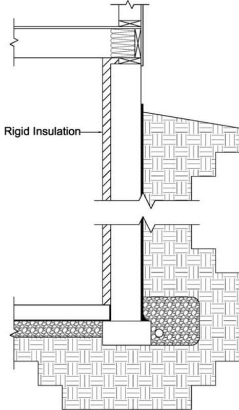
Installing foam board on the interior of the foundation provides a continuous layer of insulation. This limits thermal bridging yet makes running utilities difficult. Due to flame spread requirements, continuous foam board must be covered except for some foil-faced products.
