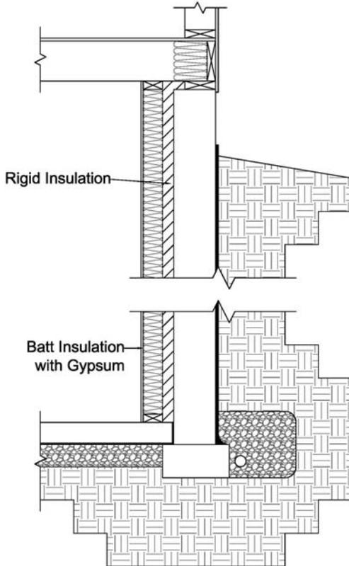
Combining continuous and cavity insulation systems offer a highly efficient basement wall. By installing a stud wall on the interior of the continuous insulation board, a finished system is provided. Thermal bridging is limited by the continuous layer but still is present. Thickness of the system becomes an issue.
