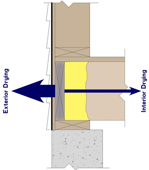
**Figure 3: Rim joist w/interior foam insulation**
