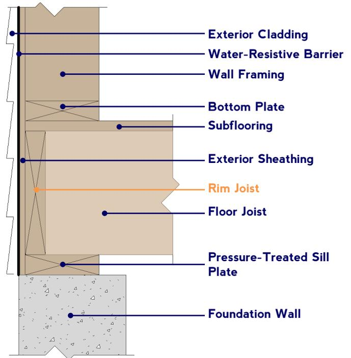
Figure 1: Uninsulated rim joist assembly
