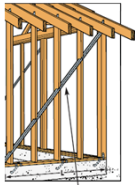
1x4 diagonal bracing or approved metal strap device. Engineer CWR, RCWB and WDW/NSC.
